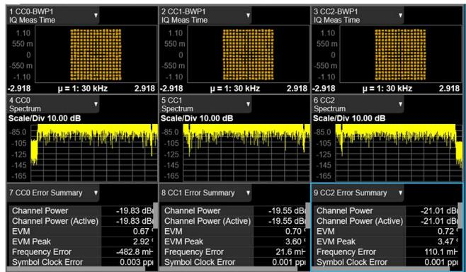
3CC x 100MHz 5GNR TDD TM3.1a EVM at 4.7GHz
