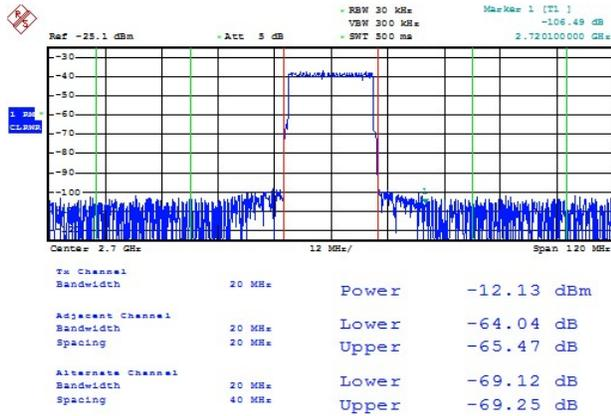
20MHz LTE RF Output at 2.7GHz
